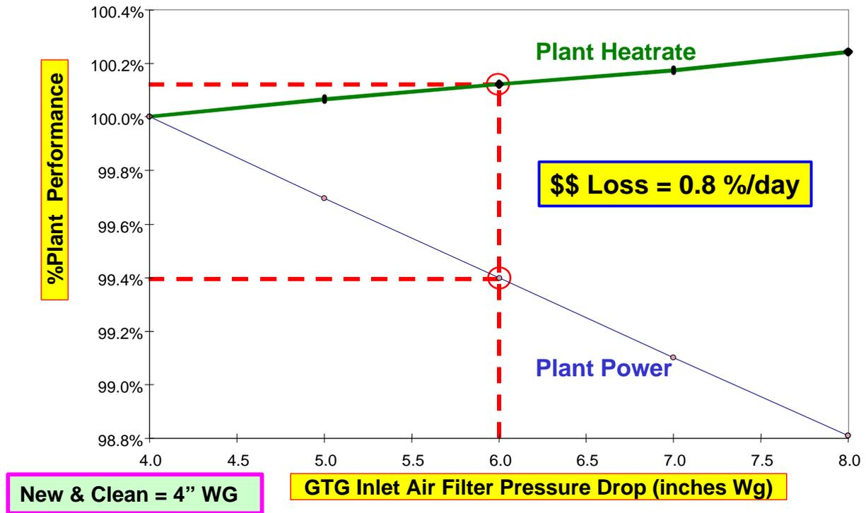
Figure 23 : Effect of GTG Inlet Air Filter Pressure Drop on the CCPP Performance and estimated daily revenue loss
