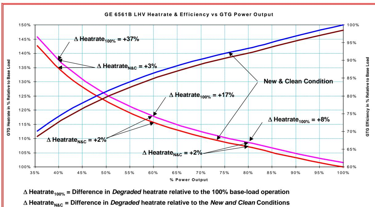
Figure 22 : Performance of a GE 6561B GTG due to a 5°C temperature rise in the compressor exit relative to the base-load/new & clean conditions.
